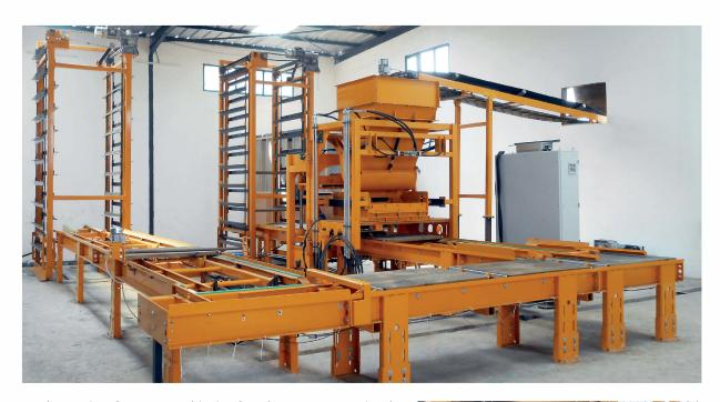
Production line for concrete blocks, foundation stones, palisade blocks, curbstones, paving stones and shallow channels, designed to meet the needs of the manufacture
