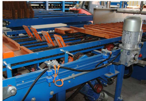
← Curing magazine unloading side and self-propelled carriage with extractor in the background.
