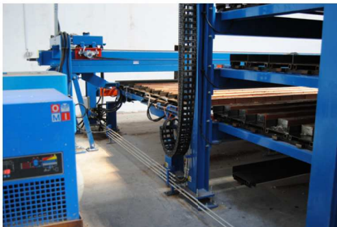
← Curing magazine unloading side and self-propelled carriage with extractor in the background.
