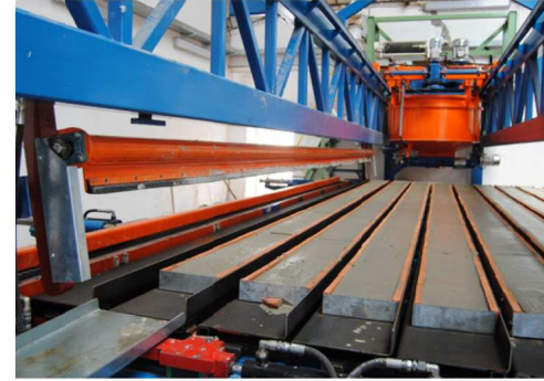
← The self-propelled batching carriage, on its own overhead track.
