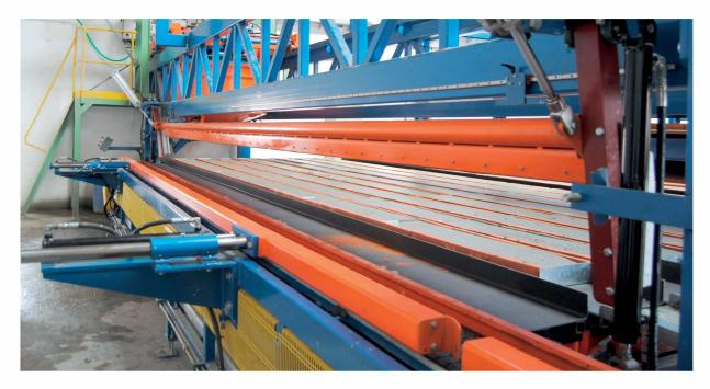
Brickbeam is designed to produce brick-concrete lattice girder beams and lintels in semi-automatic or fully-automatic process. The modular system of the Brickbeam allows various combinations and production capacity. From fresh concrete to cured concrete element Brickbeam represents the "State of Art" of industrial facility for the precast producers and furnaces.
