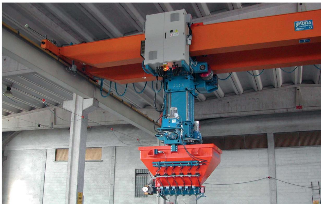
Innovative multi-purpose processing machine. KOALA can be used as lifting winch, concrete dosing system, concrete compacting and scrapping system, smoothing device and cleaning and oil release application Koala is designed to be installed in existing bridge crane and several tools are available as option.
