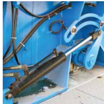
Mixer gate operation with hydraulic power pack
