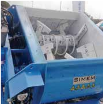
Simem own Twin shaft Mixers from 1m3 to 9m3 batch size.
