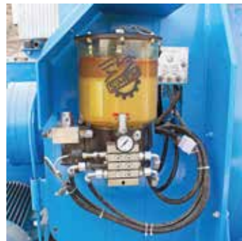
Automatic greasing system for twin shaft mixer
