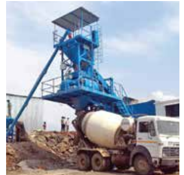
Cantilever design for easy vehicle movement
