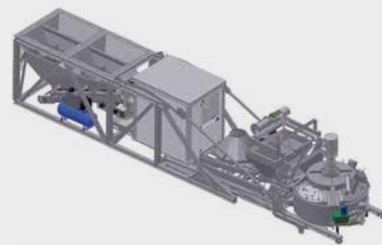
1. AGGREGATES BINS CONTROL CABIN MIXING UNIT
