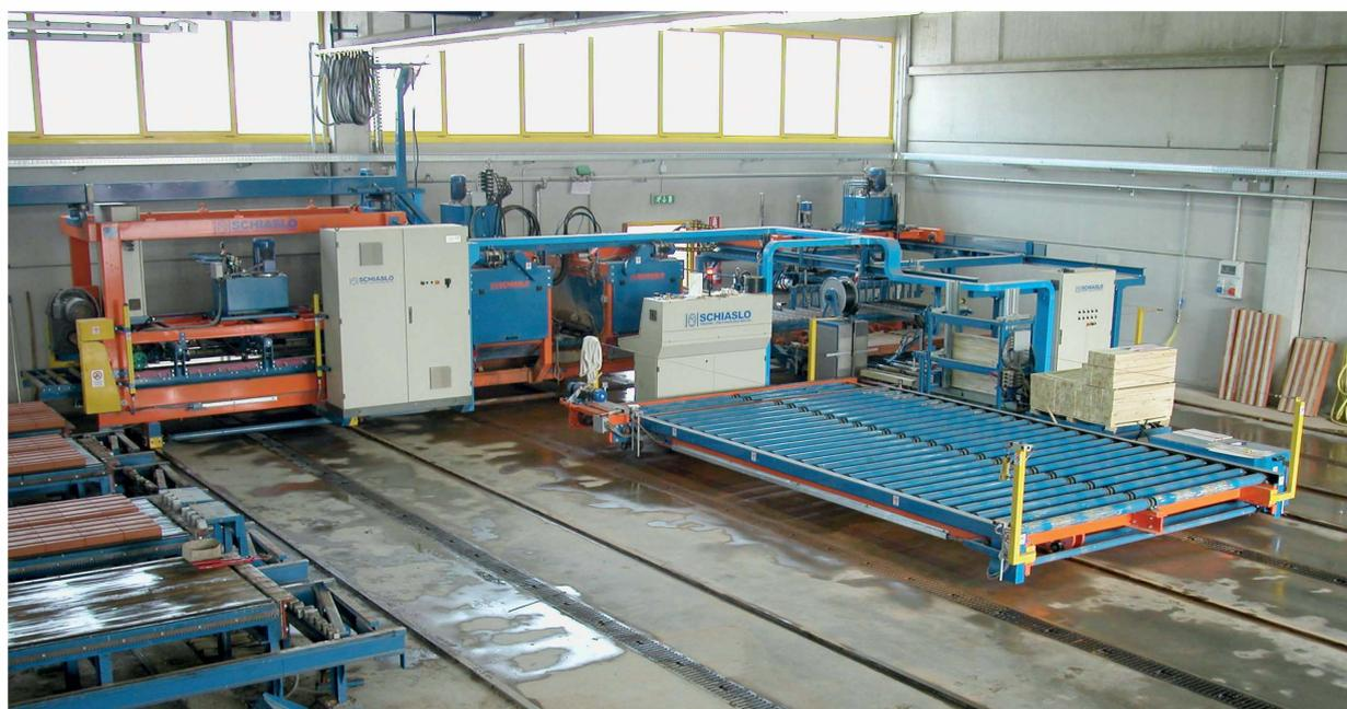
Elephant represents the "State of Art" of the industrial facilities designed to produce prestressed concrete lintels with clay-bricks. The system includes the patented "Elephant" pulling, cutting and packaging device designed to provide packed and stacked lintels without any need of manual operation. Elephant can reach massive output capacity with a reduced crew. High quality products are produced thanks to high sophisticated dosing, compacting and cutting devices.
