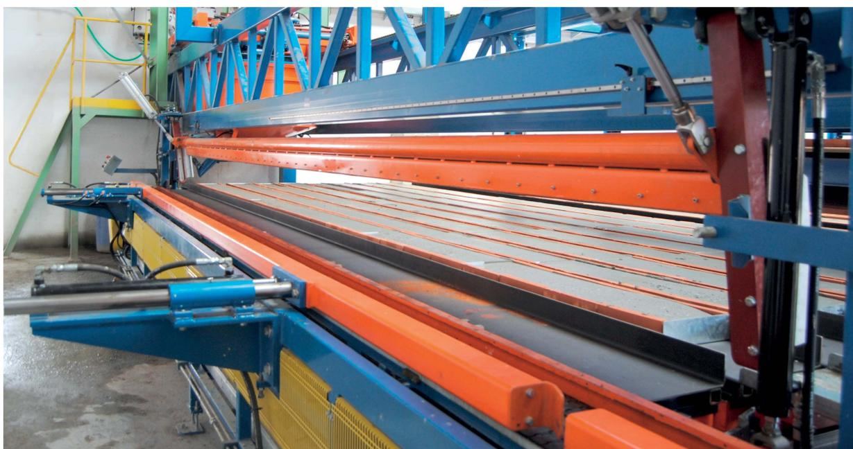
Brickbeam is designed to produce brick-concrete lattice girder beams and lintels in semi-automatic or fully-automatic process. The modular system of the Brickbeam allows various combinations and production capacity. From fresh concrete to cured concrete element Brickbeam represents the "State of Art" of industrial facility for the precast producers and furnaces.
